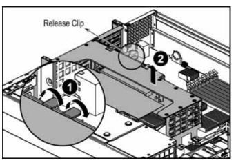
Do not touch the contacts on the bottom part of the expansion card. Touching the contacts can cause electrostatic damage to the card.
